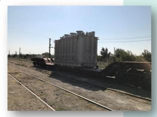
General quantity of Transformers were 2 pieces, each of which weighed 86,4 TON and with dimension 6324mm x 2702mm x 3967mm.
