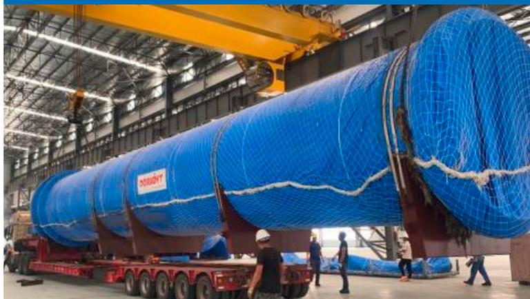
Topline Express Logistics (TEL) in China have successfully transported 2 units of dryer drum shells and their accessories from the manufacturer's premises in Shandong Province to Qingdao Port. Each unit weighed 67,000kg and measured 24.90 x 4.15 x 4.35m. The biggest challenge for TEL was a under-construction flyover that the units would have to pass under on the way to the port.
