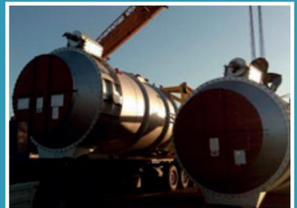
Goodrich Central Asia and former members Aryamasir have been involved in the door-to-door movement of 3 x EGPHE units, each weighing 19,500kgs and with dimensions of 7.850 x 3.397 x 3.790m.
