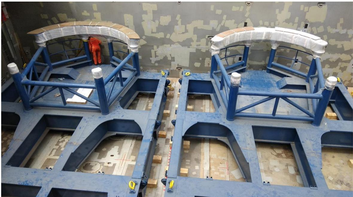
Lashed and secured inside the ship
