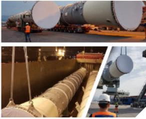
Delta Maritime in Greece are pleased to share details of a recent large project they have handled involving heavy process equipment shipped to Baku, Azerbaijan. The units measured 65m in length with a 5.5m diameter and weighed 200tns.
