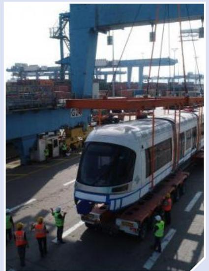
The cargo arrived from Tianjin to Haifa and was discharged directly onto extendable low-bed trailers which then transported the units to the assembly site in the Tel Aviv region. Kamor Logistics provided the local services in Israel of clearance, land transport and discharge at the receivers' premises.
