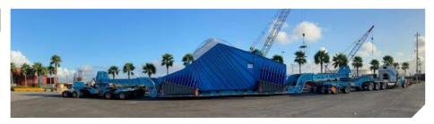
chains in the vessel hold. After 36 days on the water, the ship arrived at the Port of Houston and the pieces were unloaded and onto truck trailers for the road transportation. Step deck trailers were used in order to ensure clearance throughout the journey.
